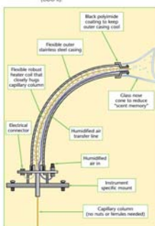
Figure 2. Internal design of the Olfactory Detector Outlet (ODO II).
