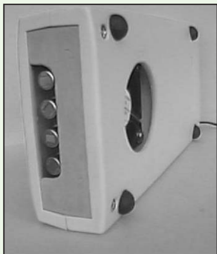
Plate 1: Photograph of a four sensor nose – dimensions: 5 x 10 x 20 cm
