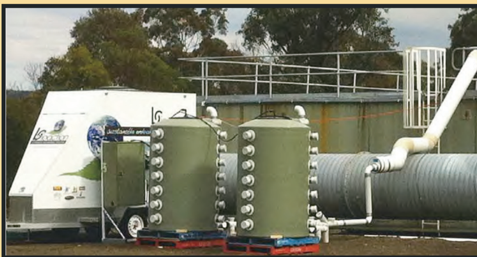
Figure 3: Odour was measured at varying depths in two experimental biofilters (Bioaction Pty Ltd). Ports for air sampling at varying depths can be seen on each filter vessel. The E-Noses were located inside the trailer at left. Odour was piped to the filters from a fertilizer plant at right (Bell and Botham 2011).
